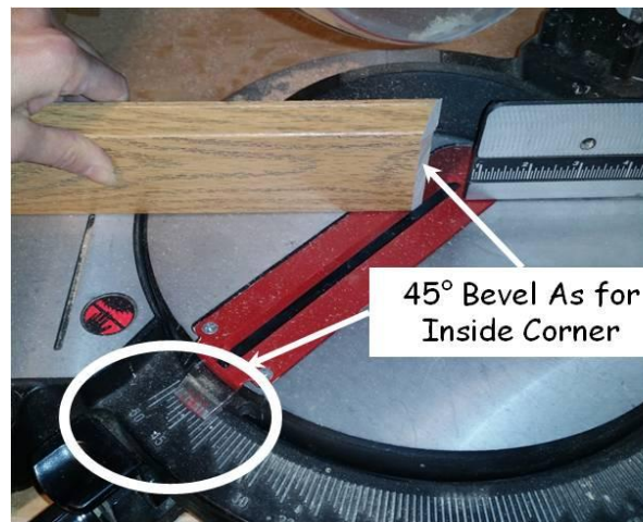
Figure 19-5. Base Trim Bevel Cut.
