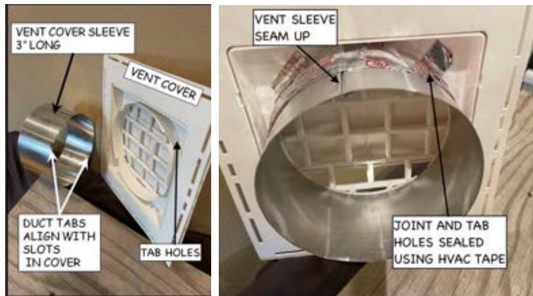
Figure 10-2 – Range Vent Cover Sleeve Assembly
