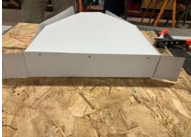
Figure C-12. Plenum With Bottom Secured.
