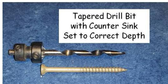
**Figure 17-2. Setting Tapered Drill Bit to Correct Depth.**
