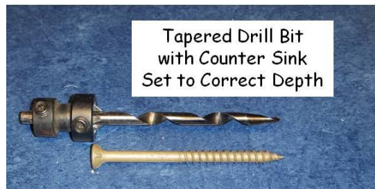
Figure 17-2. Setting Tapered Drill Bit to Correct Depth.
