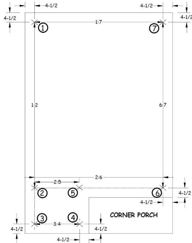
**Figure 1-2. Sill Plate Layout with Corner Porch.**
