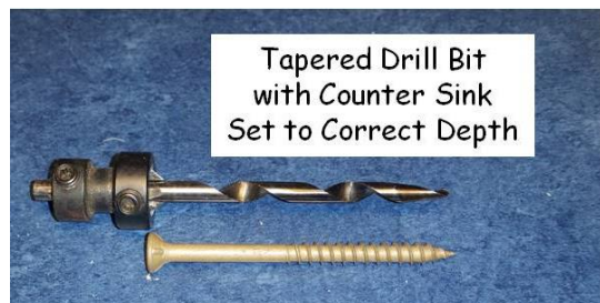
Figure 17-2. Setting Tapered Drill Bit to Correct Depth.
