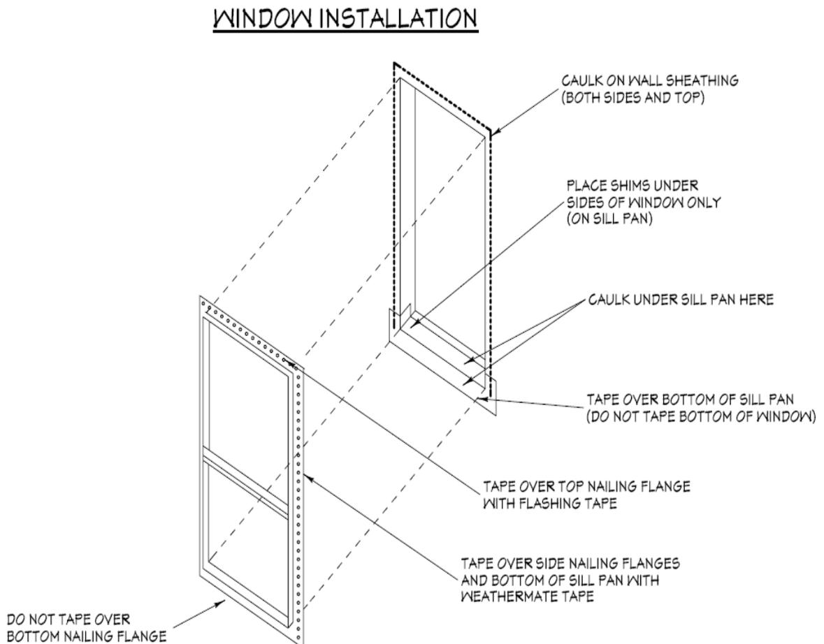
**Figure 9-1. Window Installation**
