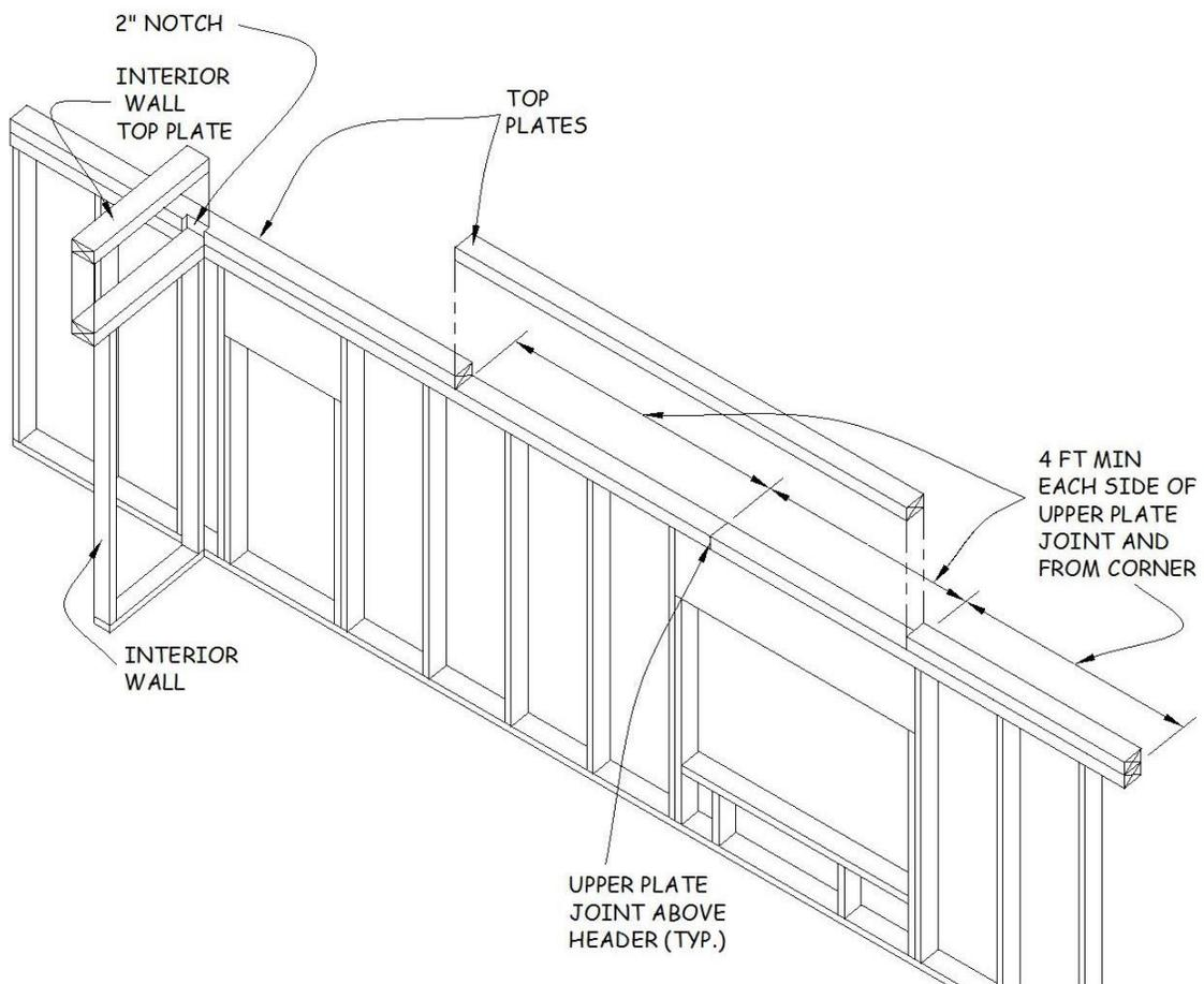
Figure 5-3. Exterior Wall Top Plate Installation.
