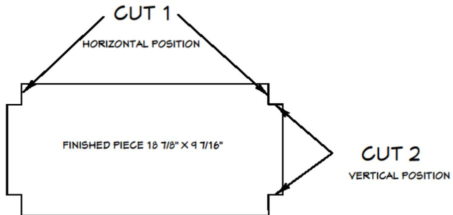
**Figure 2-2. Foamboard notches.**
