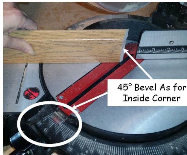
Figure 19-2. Base Trim Bevel Cut.
