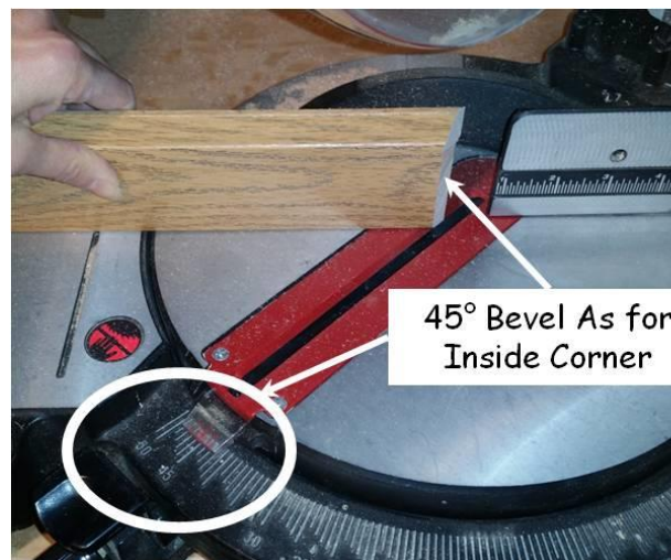
Figure 19-1. Base Trim Bevel Cut.
