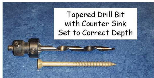
Figure 17-2. Setting Tapered Drill Bit to Correct Depth.
