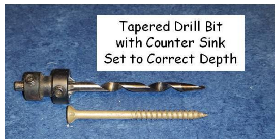
Figure 17-2. Setting Tapered Drill Bit to Correct Depth.
