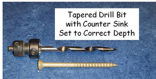
Figure 17-2. Setting Tapered Drill Bit to Correct Depth.
